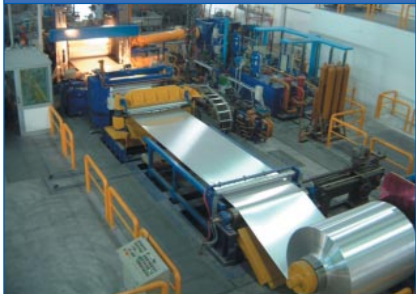
The first Prezezzi TT1000 continuous casting line at Profilglass (Fano, Italy)
